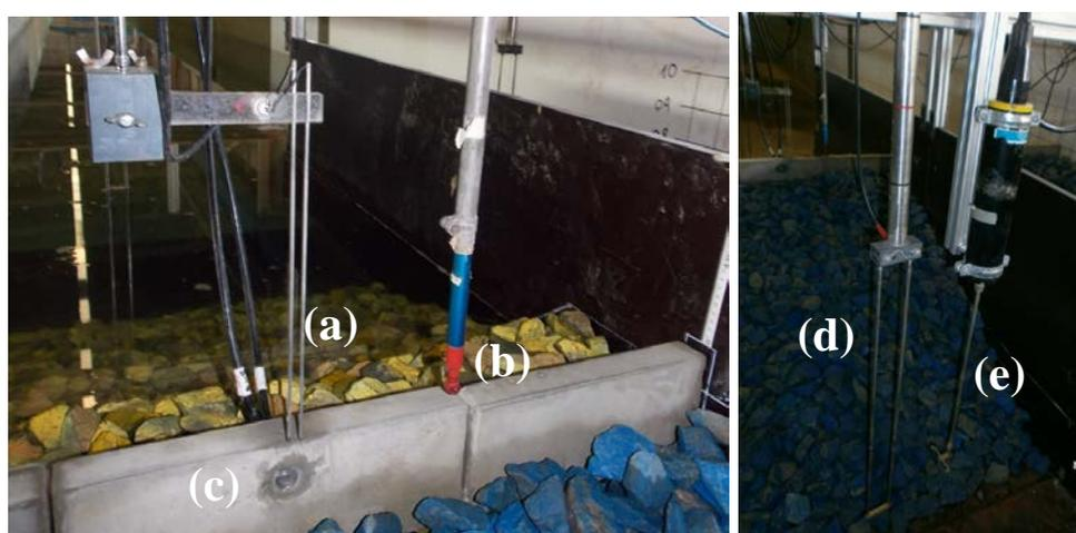
*Figure 2.9: Exemplary arrangement of overtopping wave gauge (a), propeller current meter (b), pressure sensor (c), normal wave gauge (d) and ADV current meter (e) in tests at TU-BS*
