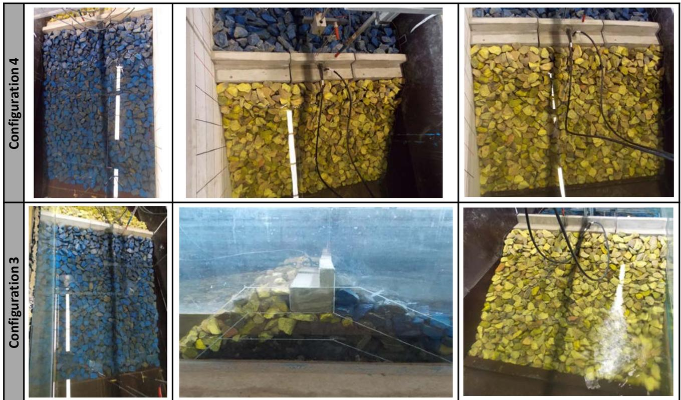
Figure E 11: Damage of configurations 3 and 4 due to solitary wave with  $H=0.050\text{ m}$  (Test 20150106\_01)
