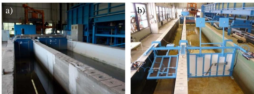
Figure 2.1: Twin-wave flume at LWI, TU-BS with 1.0 m wide channel (left) and 2.0 m wide channel (right) with: a) wave maker, b) bore gate
