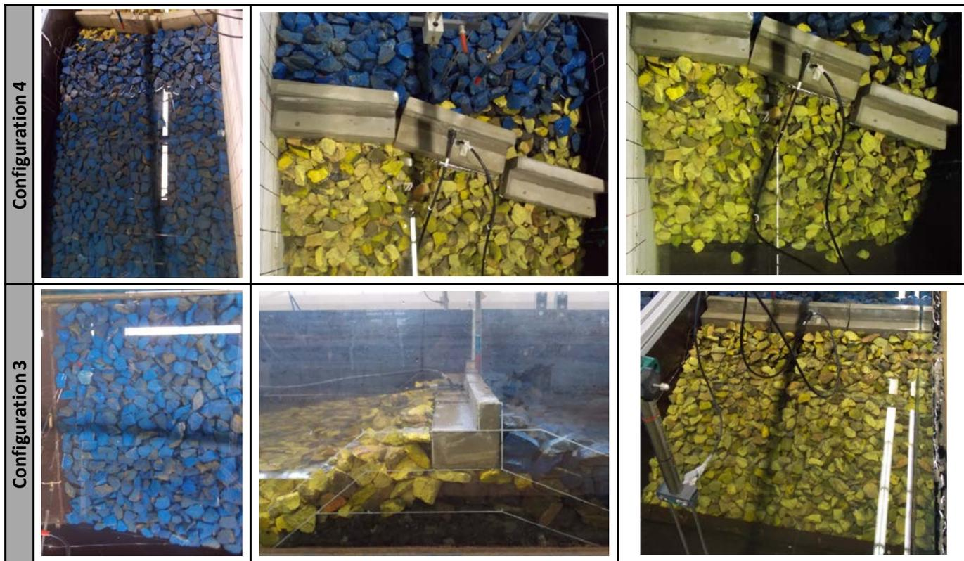
Figure E 13: Damage of configurations 3 and 4 due to solitary wave with  $H=0.100\text{ m}$  (Test 20150107\_01)
