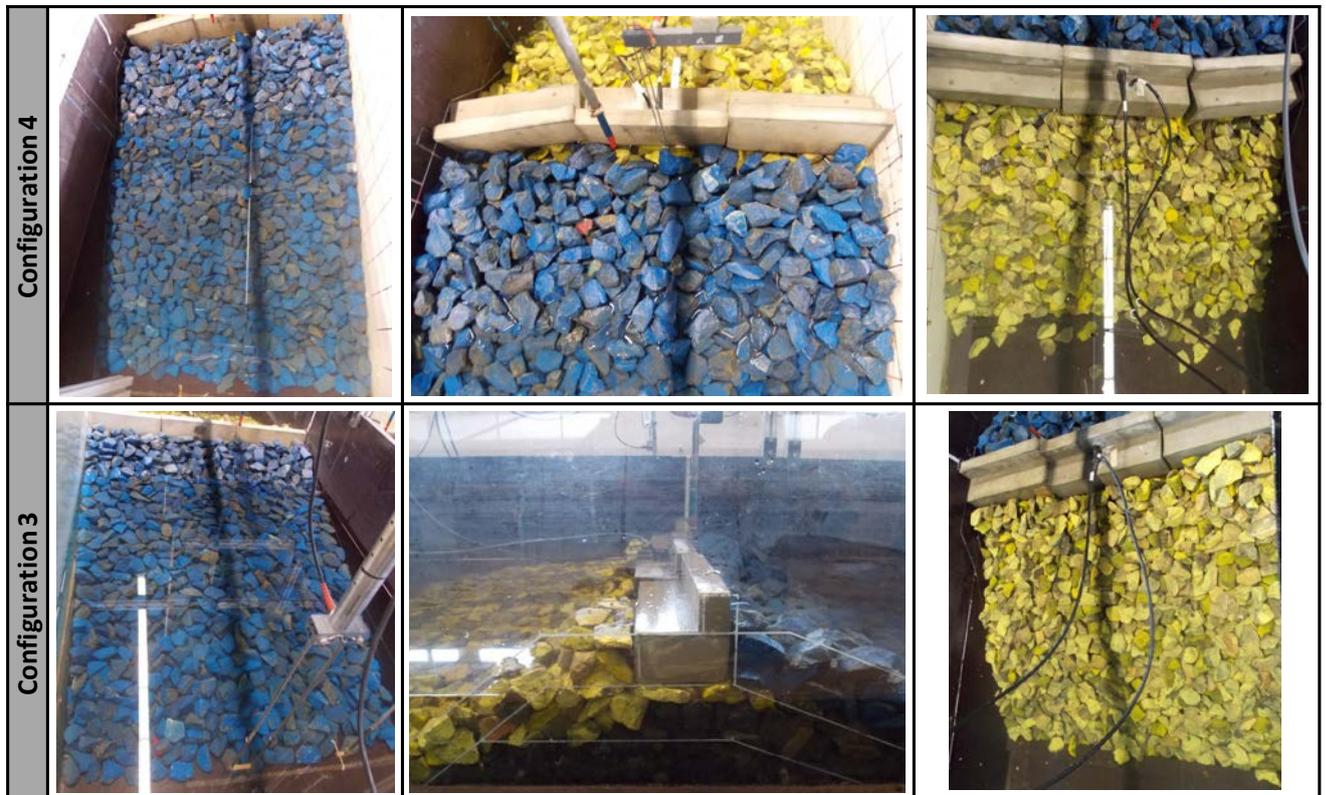
Figure E 14: Damage of configurations 3 and 4 due to solitary wave with  $H=0.125$  m (Test 20150108\_01)
