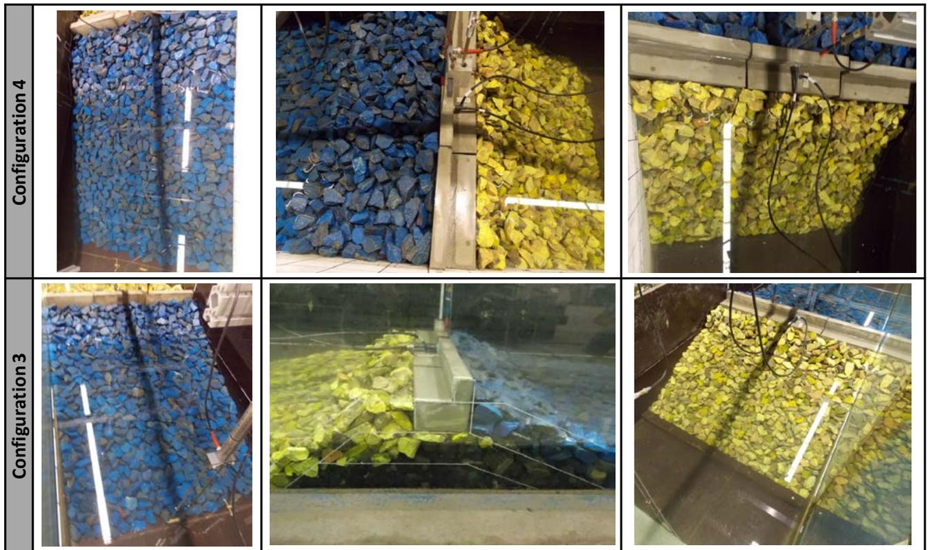
Figure E 12: Damage of configurations 3 and 4 due to solitary wave with  $H=0.075$  m (Test 20150106\_02)
