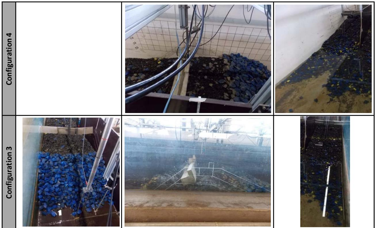
Figure E 3: Damage of configurations 3 and 4 due to tsunami bore with  $h_0=0.85$  m and  $h_1=0.20$  m (Test 20140721\_03)
