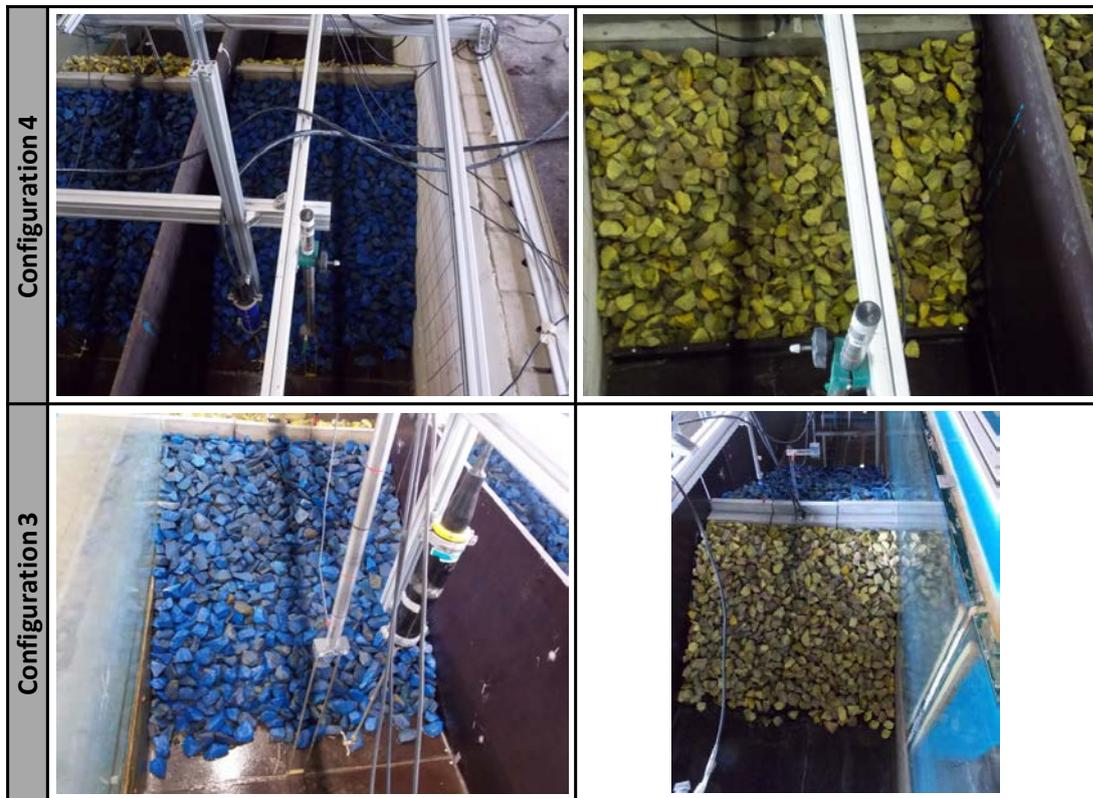
*Figure E 2: Damage of configurations 3 and 4 due to tsunami bore with  $h_0=0.80$  m and  $h_1=0.20$  m (Test 20140721\_02)*
