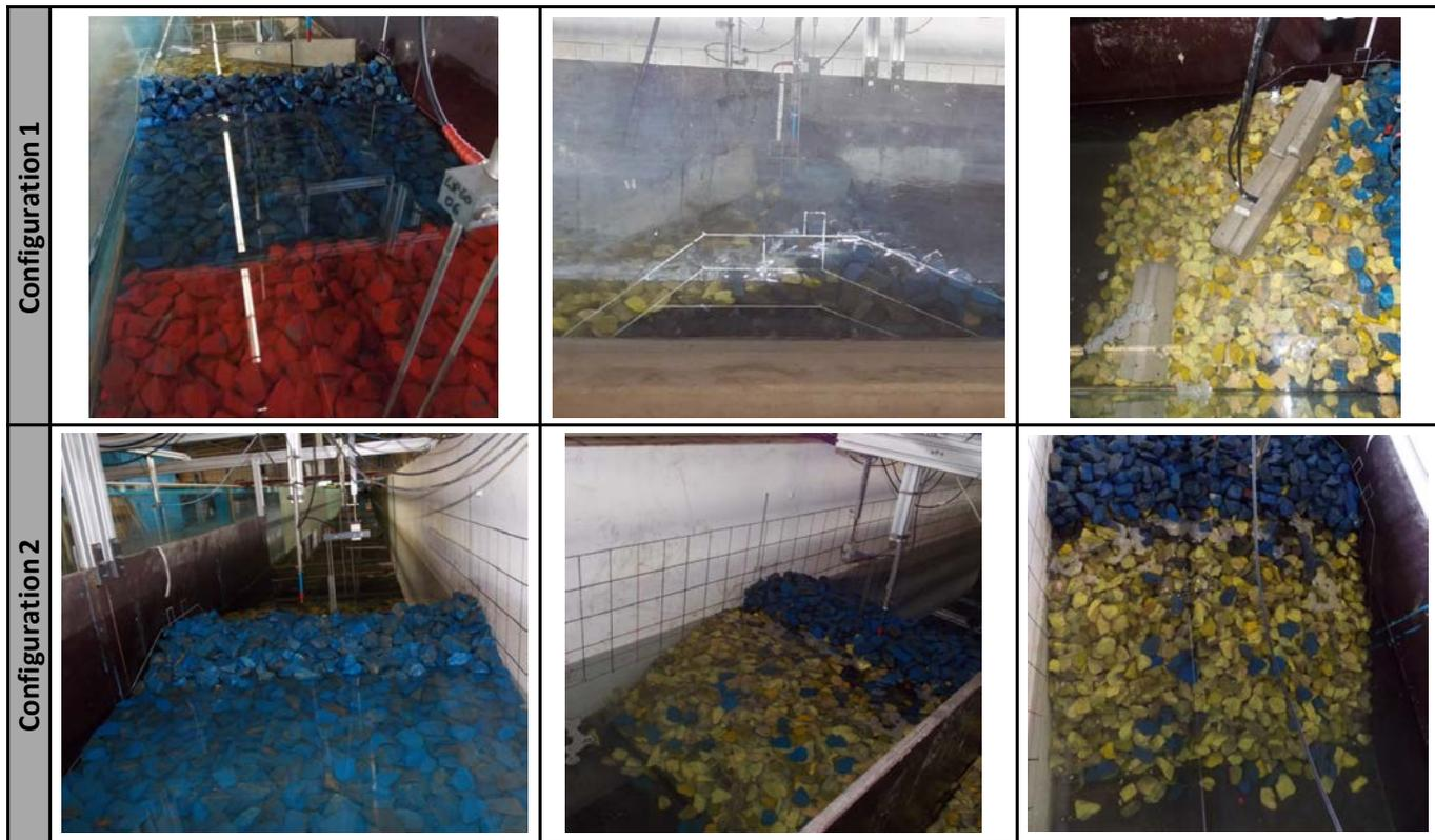
Figure E 10: Damage of configurations 1 and 2 due to solitary wave with  $H=0.150$  m (Test 20140807\_03)
