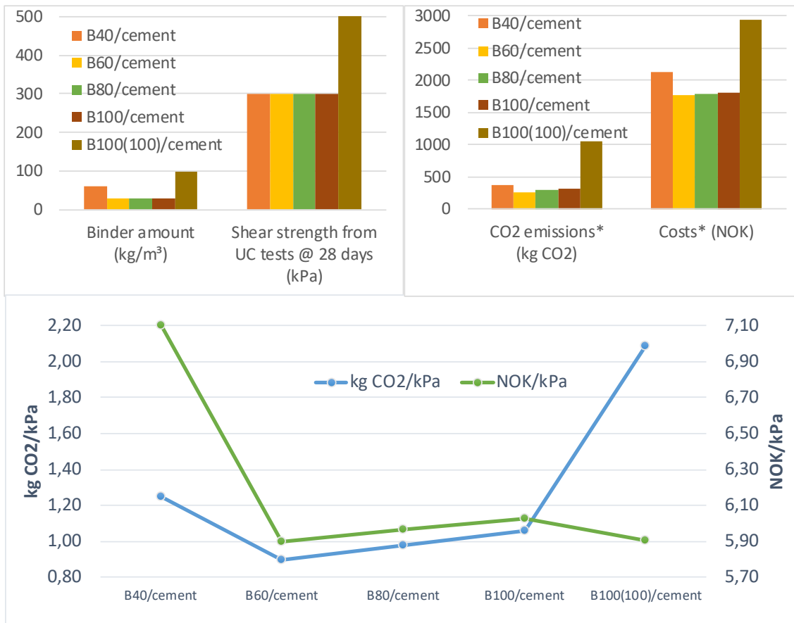
Figure 1 kg CO 2 and NOK per unit shear strength (kPa) for five binders (B40, B60, B80, B100) and cement.
