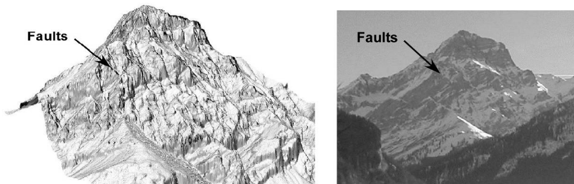
Figure 40: HRDEM and picture of the west face of the Grand Muveran Mountain (Switzerland). Picture from Jaboyedoff et al. (2007). Source of the ALS dataset: MNT MO/MNS.
