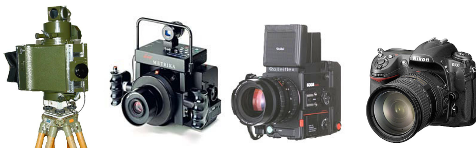
Figure 5 : Typical sensors for terrestrial photogrammetric surveys in historical order (left to right): Phototheodolite Zeiss Photheo, Linhof Metrika, Rolleiflex 6006, and Nikon D300
