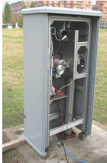
Figure 142 : Automatic probe inclinometer (courtesy of Ing Lollino, CNR-IRPI Italy).
