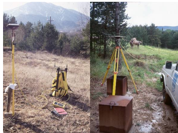
Fig. 6. Examples of Vallcebre monitoring points with different antenna set-up methods: telescopic pole (left); tripod with optical plummet over an inclinometer borehole (right).
