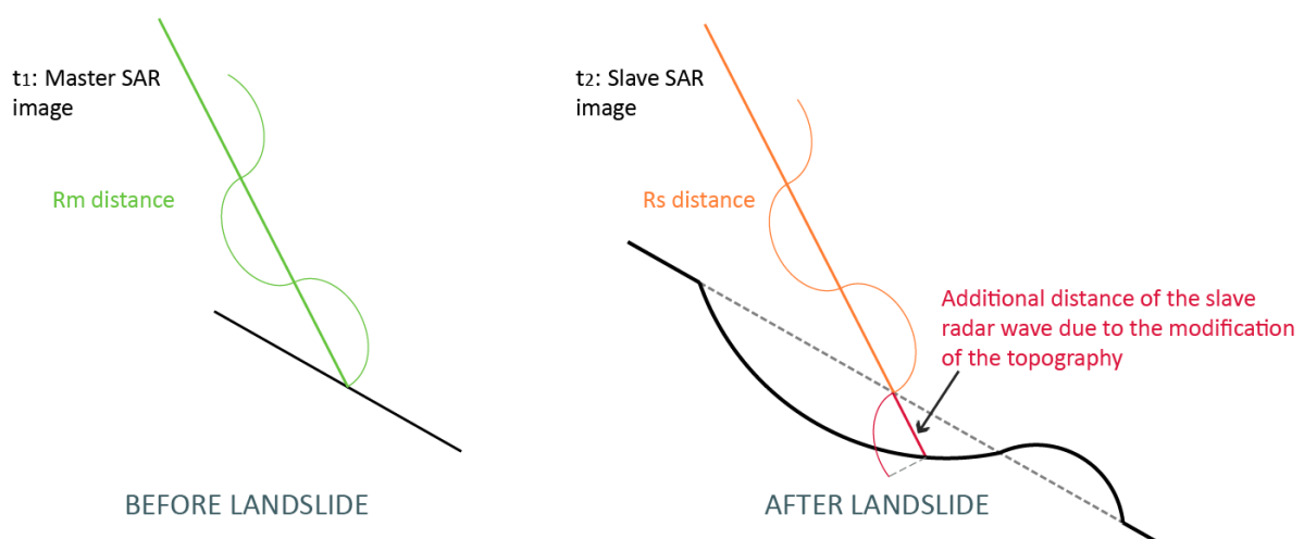
Figure 65 : Influences of a slope deformation on the phase decay. The way of the slave SAR image is longer than the way of the master SAR image, due to the rotational landslide (Michoud et al., 2009, modified).
