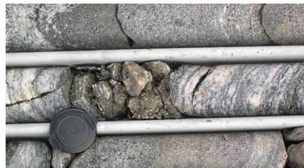
Fig. 5. Drilling core at 34 m depth at the middle borehole at Åknes, showing a crushed and brecciated zone with silt and clay, representing the upper sliding zone. This sliding plane is also documented by displacement in DMS™ column (Differential Monitoring of Stability, in place instrumentation).
