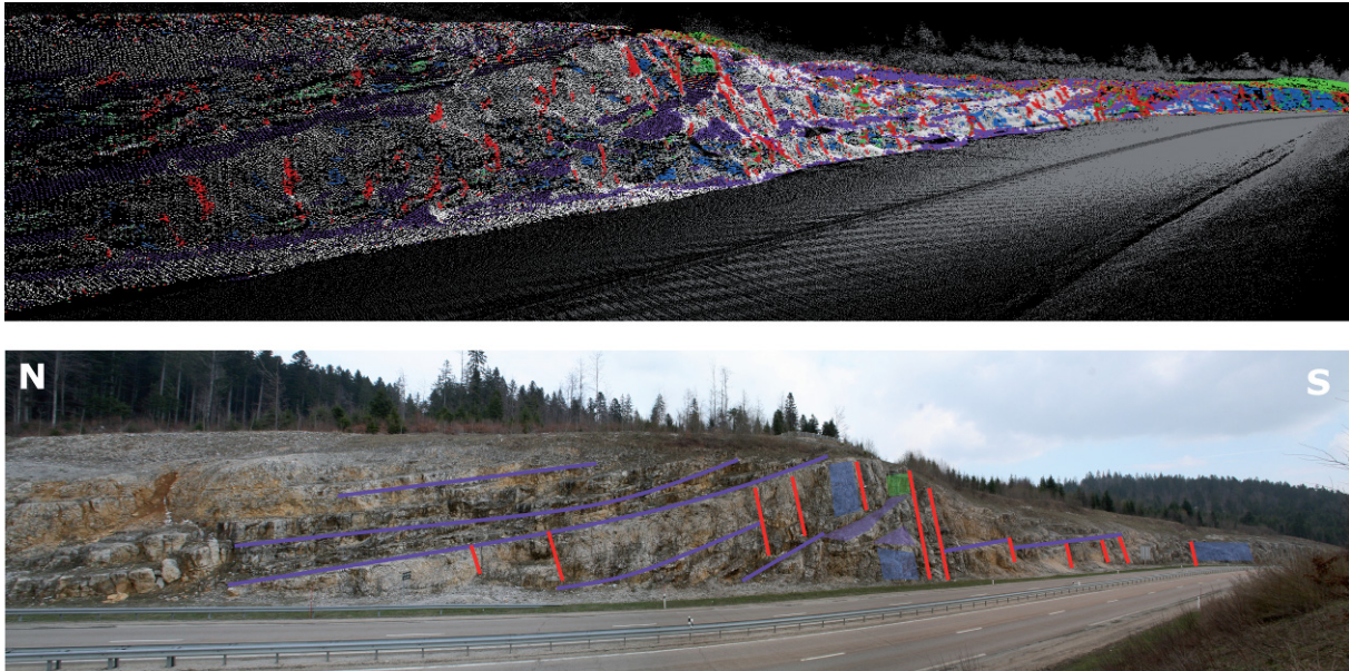
Figure 160 : Up. Point cloud acquired thanks to LYNX Mobile Mapper, highlighting main discontinuity sets. Low. Corresponding outcrop on field. (Carrea et al., 2010)
