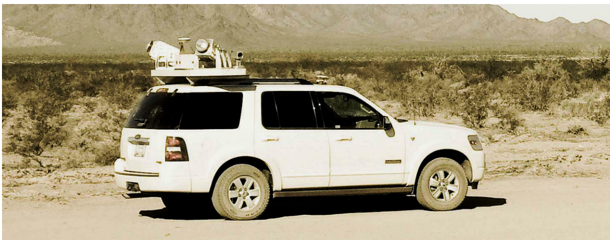
Figure 161 : LYNX Mobile Mapper apparel on the roof of the car. (Optech website, 2010. Available at http://www.optech.ca/press_LYNX_Release.htm )
