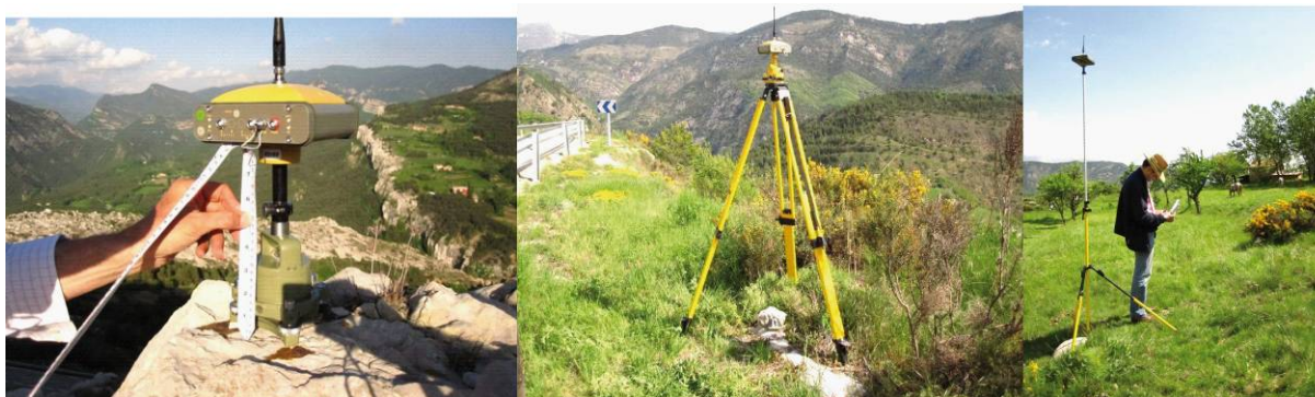
Figure 153 : Different antenna set-up: antenna directly over a rock outcrop; setting-up with tripod and optical plummet; antenna over a telescopic pole.
