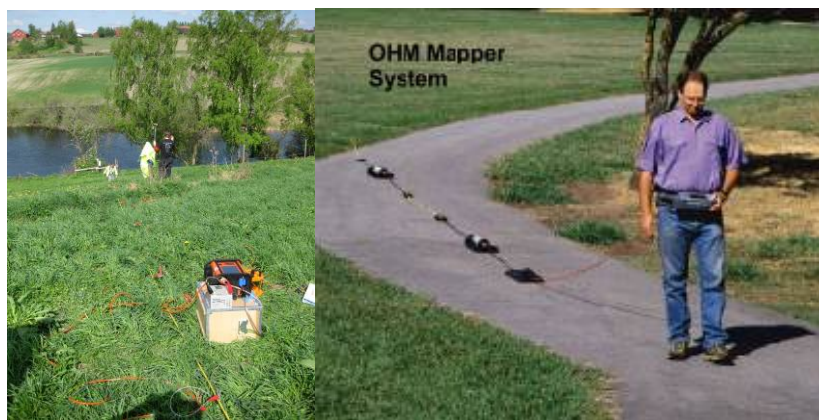
Figure 108 : Electric resistivity tomography (ERT). a) Electrodes planted in the ground are linked together with electrical cables to an electronic console (courtesy of S. Bazin). b) An alternative system can be towed (picture from www.geometrics.com )
