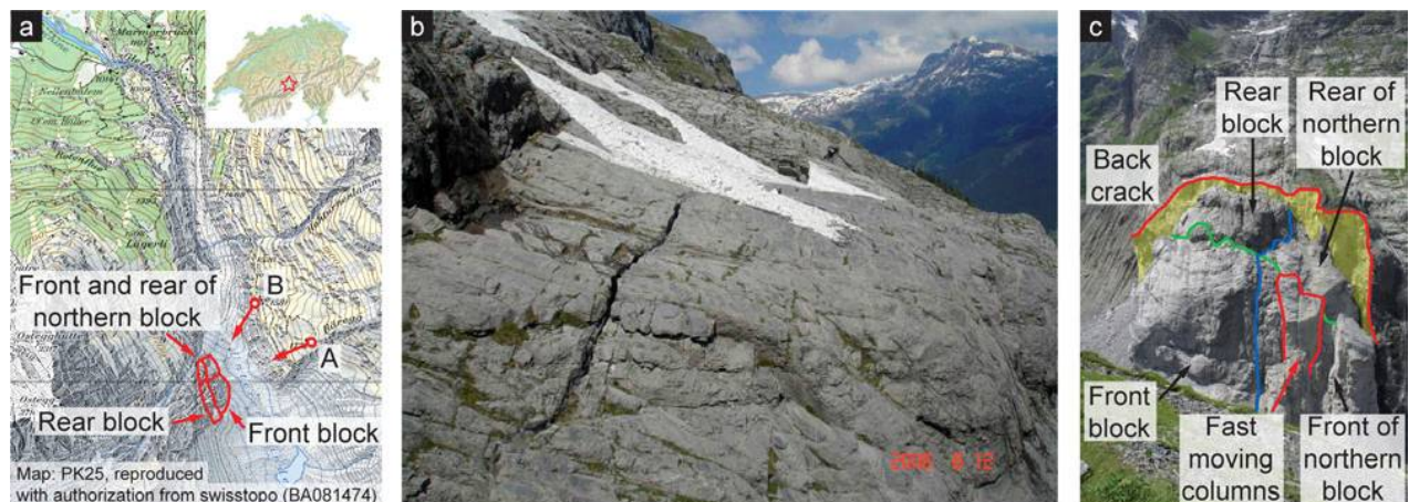
Fig. 1. a) Situation map of the Eiger rockslide; b) Picture of the back-crack at the beginning of the monitoring campaign (Picture: Geotest AG); c) Frontal view of the Eiger rockslide showing the division of the spur into a front and a rear block separated by a steep middle fracture (green line) and the northern rear and front blocks are separated from the main blocks by a bedding plane (blue line).
