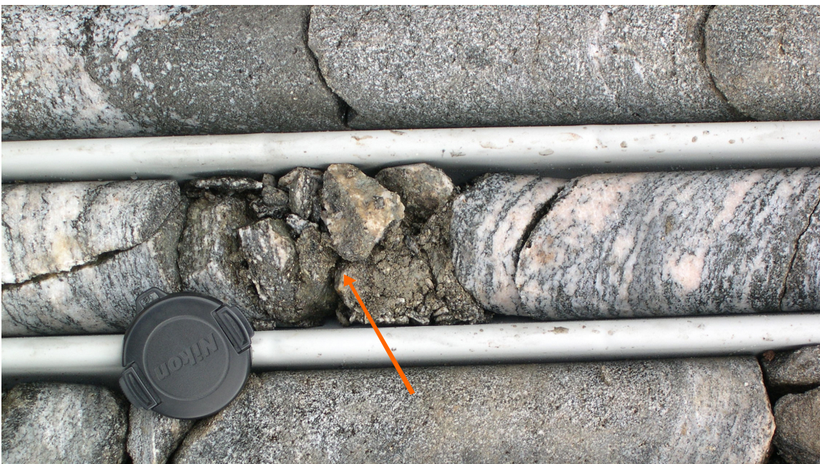
Figure 155 : Core logging in Åknes. Middle borehole, 32 m depth: crushed and brecciated zone with silt and clay which represents the upper sliding zone, also documented by displacement in DMST TM column (Differential Monitoring of Stability, in place instrumentation).
