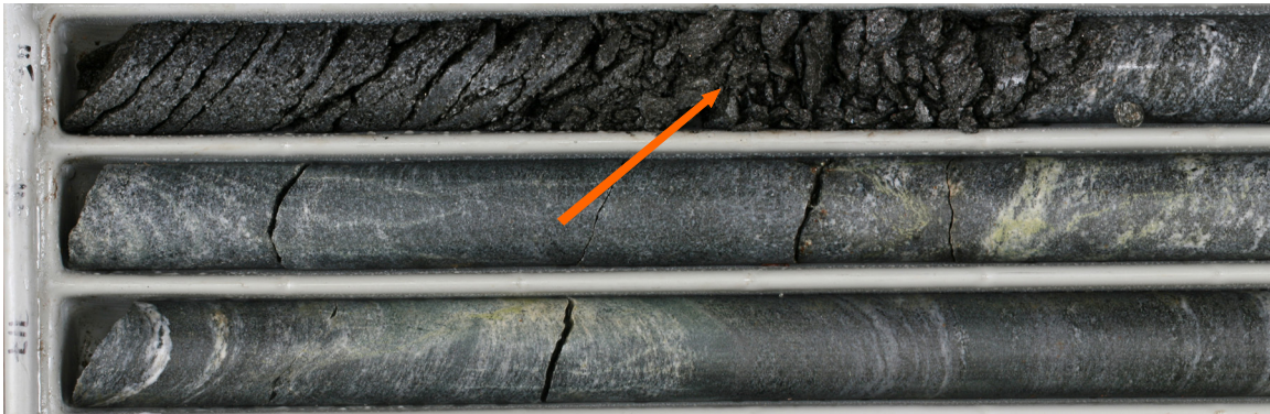
Figure 154 : Core logging in Åknes. Lower borehole shows a crushed zone at 115 m depth, possible representing a sliding zone.
