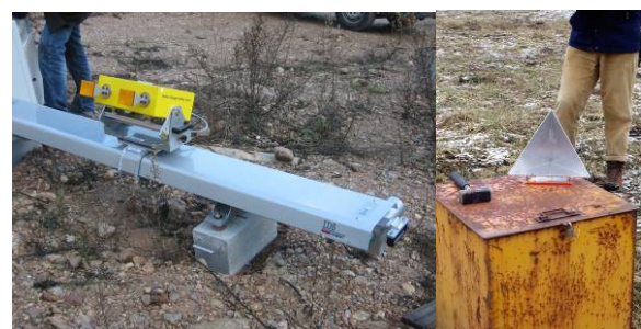
Fig. 13. The IBIS-L-IDS GBSAR system installed in front of the Vallcebre landslide by the Institute of Geomatics for the first tests. A number of mini-corners (right) were deployed in the scene.
