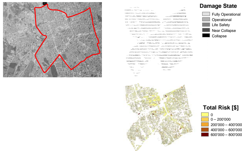
Figure 6: Results of a risk assessment utilizing generic BPN risk models and GIS data bases.
