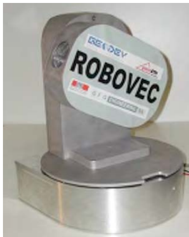
Figure 13 - Prototype of the ROBOVEC. The laser distance meter is enhanced with a bi-axial modular robotization (Manetti & Steinmann, 2007).
