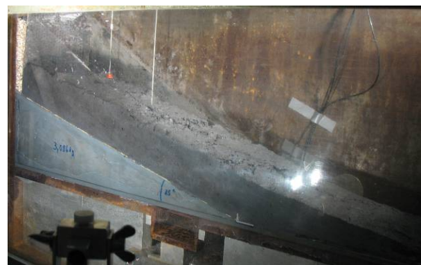
Figure 19 - Failure that occurred during the consolidation phase for unsaturated clay with an initial water content higher than the optimum water content (about 18%).
