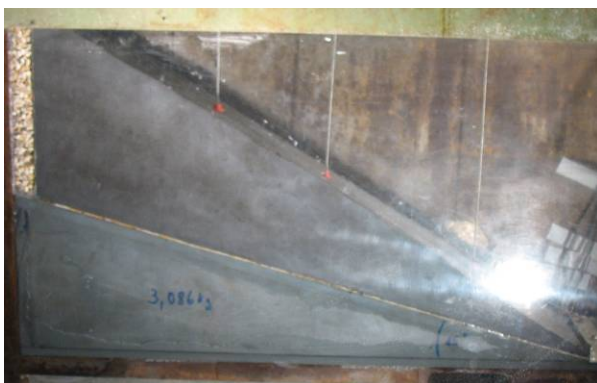
Figure 18 - Start of the consolidation phase for unsaturated clay with an initial water content higher than the optimum water content (about 18%).
