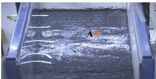
Figure 19 - Initial test conditions (height = 26 cm, width = 60 cm, length = 91 cm) and observation point A.
