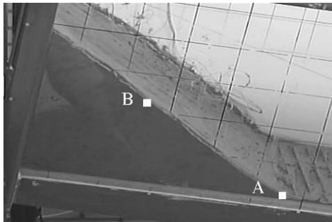
Figure 13 - Initial test conditions and observation points for the flume test on Zoelen clay.
