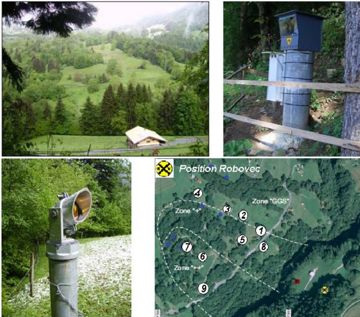
Figure 14 - View of the La Frasse landslide from the opposite side of the valley where the ROBOVEC has been installed in June 2006 (top); one of 9 geodetic prisms that have been installed on the site and a map showing the location of the targets and the ROBOVEC (bottom) (Manetti & Steinmann, 2007).
