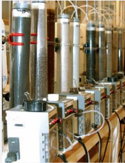
Column leaching test
